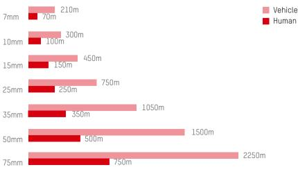
Notice:this distance is based on 17µm sensor. VCA rules: line crossing, intrusion.
