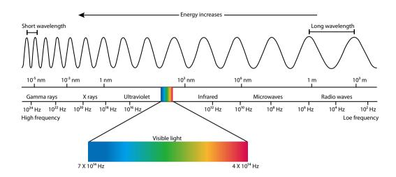
While invisible to human eyes, thermal cameras detect this kind of radiation (from wavelength 8 to  $14~\mu m$ , or 8,000-14,000~nm) and produce images (thermograms) using temperature differences. Thermography makes it possible to see the environment with or without visible light, and thus is widely used in such areas as video surveillance, fire detection, environmental control, building analyses, medical analyses, and others.
