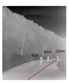
Detection, recognition and identification distance (Under 8mm lens)
